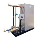
**BWXP** - Compact plate heat exchanger indirect water heater utilizes low temperature boiler water to heat domestic water. Designed to fit through a standard door opening.
